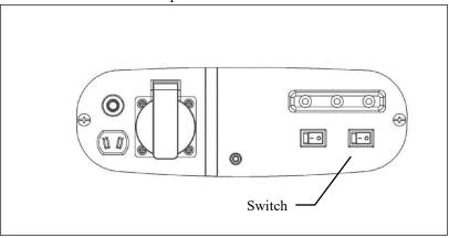
3. Turn the oil switch to "OFF" position.
